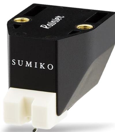
The Rainier has a simple elliptical stylus (only in relation to the higher cartridges in the series; no elliptical stylus is truly simple), and its cantilever is an aluminum pipe. Its specifications include a frequency response of 15Hz-25kHz, channel separation of 25dB at 1kHz, channel balance of 1.5dB at 1kHz, and output of 5.0mV. The range of vertical tracking force (VTF) is
